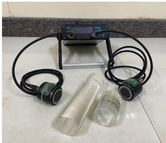
Ultrasonic Pulse Velocity Instrument with Standard Calibration Bars
